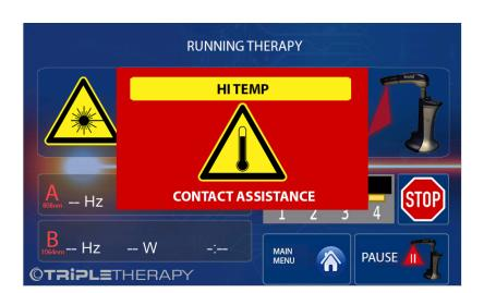
Should this occur, wait for it to cool down with the device switched on for about ten minutes and try the start of therapy again. If the problem persists contact technical support
