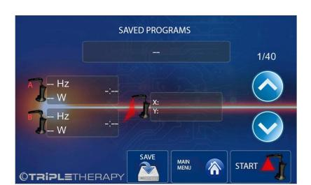
To save the therapy choose one of the 40 positions available by pressing on the icons in the shape of an arrow until you reach the desired position (by default the first position is set) and press the SAVE icon to access the virtual keyboard to type the name to be assigned to the therapy you are saving.
