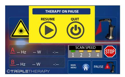
You can also stop permanently and emergency, with return to the main menu screen, the therapy running pressing on the STOP icon.
