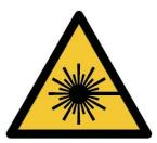
Meaning: Warning plate - Danger from laser radiation source
