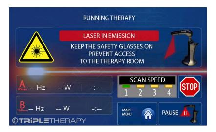
In this screen for each activated laser source are displayed the parameters set and the time countdown at the end of the emission and you can select the desired scan speed among the four available by pressing on the icons marked by numbers 1 to 4 (Speed 1 is selected by default).
