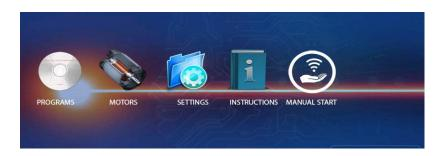
The second icon from the left, depicting an motor, allows access to this menu. So proceed by clicking on it and wait for the screen to appear ARM ADJUSTMENT AND TESTED.
