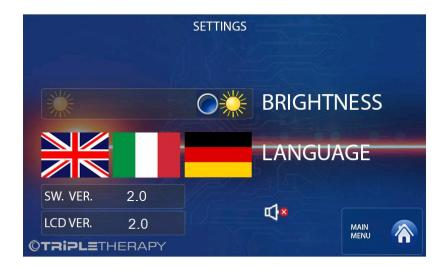
Drag the slider of the LIGHT bar' from left to right to adjust the brightness of the display from weak to stronger.
