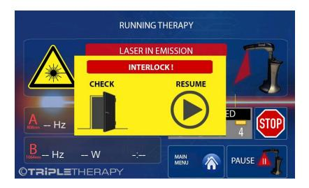
To resume the therapy it is necessary to close the door and press on the icon RESUME. The following controls are active during the duration of the broadcast
