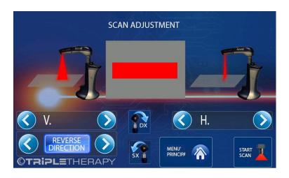
Acting on the arrow-shaped icons of the fields V. and H. you vary the scanning area respectively along the horizontal and vertical direction
