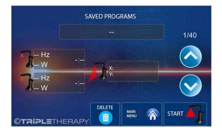
To scroll through the stored therapies press on the arrows until the therapy you want to start and confirm it by pressing the START icon, you will have direct access to the screen ARM AND HEAD ADJUSTMENT of manual mode (figure 9) from which to continue as already explained To delete a stored therapy from the list press the DELETE icon.
