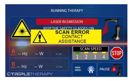
If, on the other hand, the malfunction is permanent, the pop-up **SCAN ERROR CONTACT ASSISTANCE** will appear in the main menu; the device is no longer able to execute any therapy and only the MOTORS, SETUP and GUIDE functions remain active.
